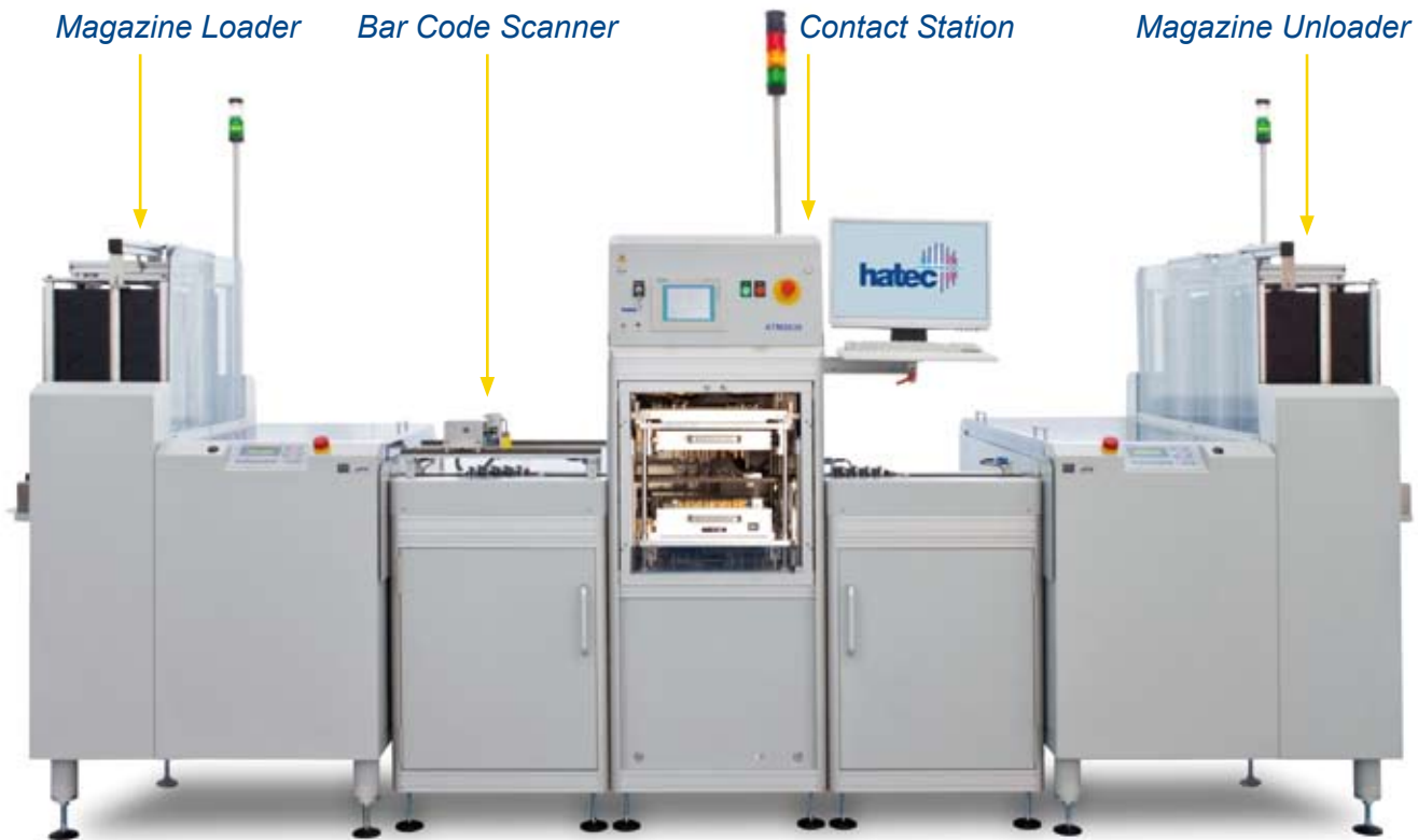
Example: ATM 2630 with loader, bar code scanner, contact station, buffer conveyor and unloader.
