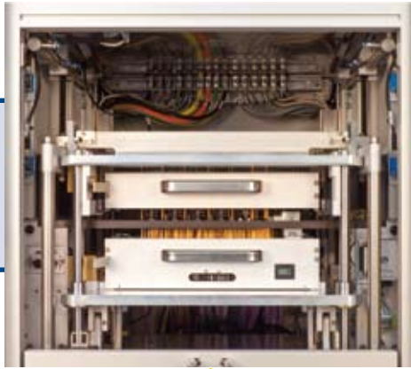
Adapter partially opened: for FCT, using long travel spring contacts
