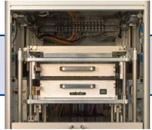
Adapter closed: In Circuit test, using standard spring contacts
